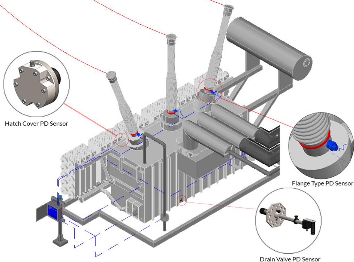
Fig. 3: Three forms of UHF PD measurement probes used in transformer monitoring
