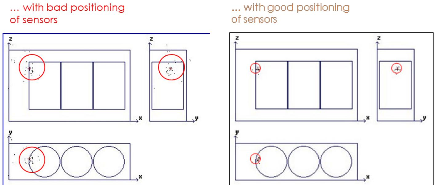
Fig 5: Illustration of the effect of bad and good positioning of sensors on the accuracy of fault location. Image courtesy of Raja Kuppaswamy. [3]
