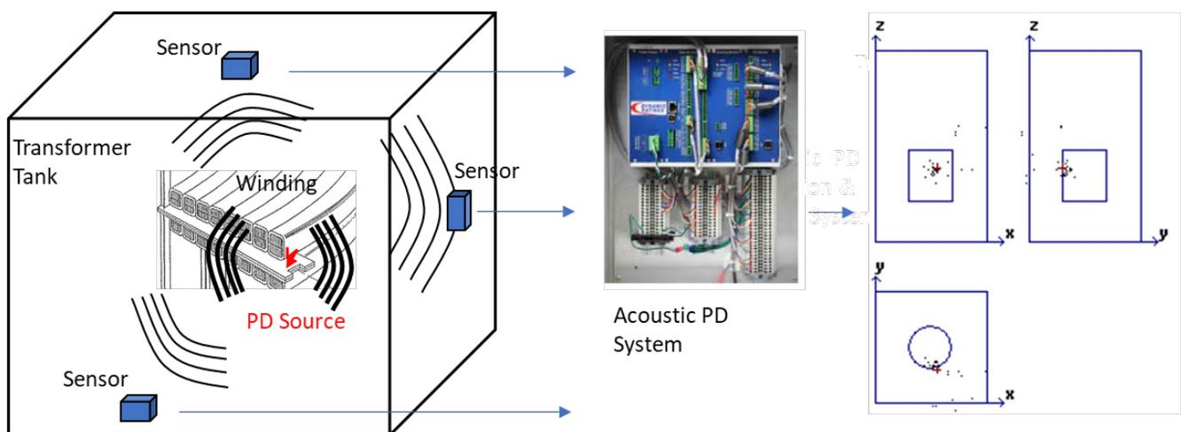
Fig 4: Principle of Ultrasonic (Acoustic) PD Measurement. Drawing (left) and screen shot (right) courtesy of Raja Kuppaswamy.
