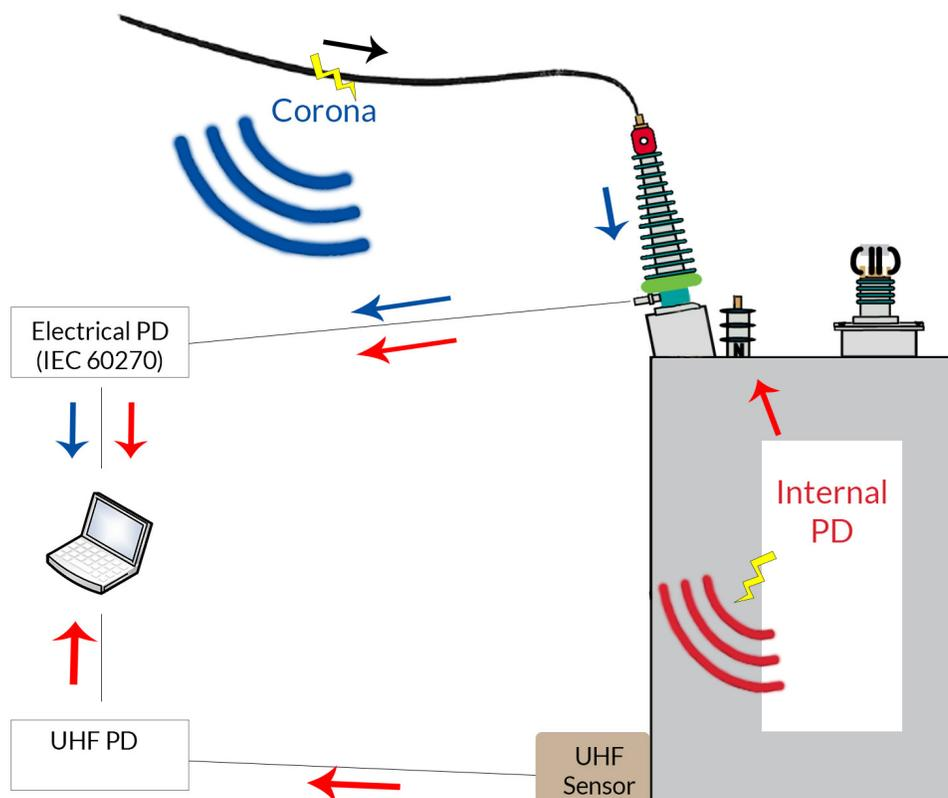
Fig. 2: Principle of UHF partial discharge measurement
